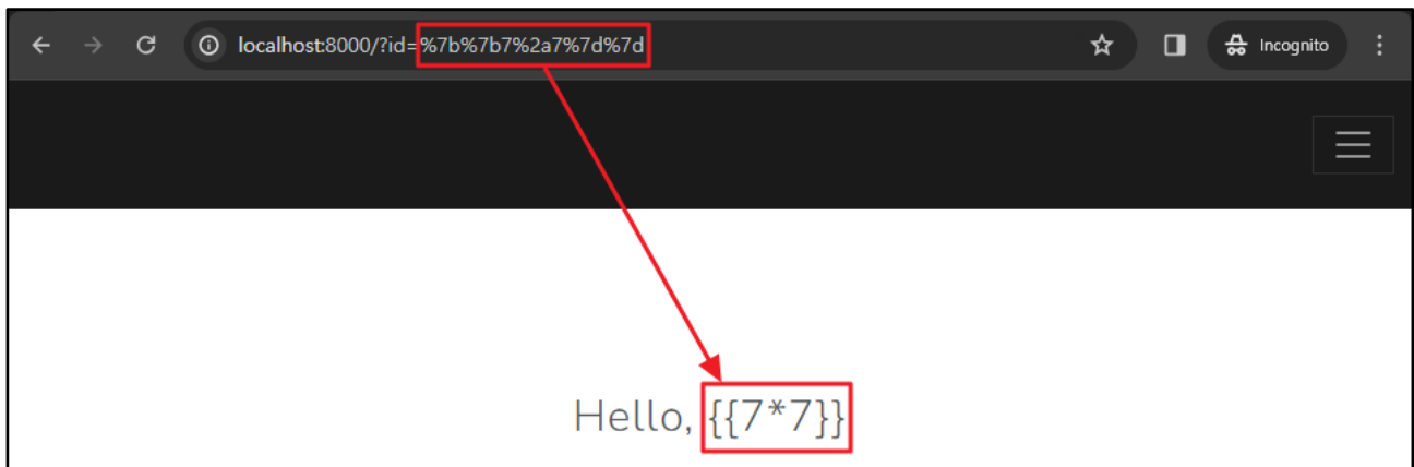
Figure 8. if {{7*7}} statement is entered in the Jinja2 Template Engine after Sanitization
